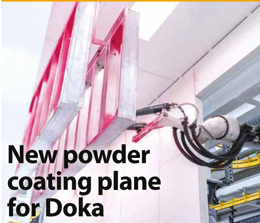
LEFT: Automatic, digital and flexible: Doka's new powder-coating plant selects the right powder application method, such as the robot hand, to suit a client's needs (image courtesy Doka) BELOW: Doka's new chief executive, Robert Hauser: more digitalisation (image courtesy Doka)
